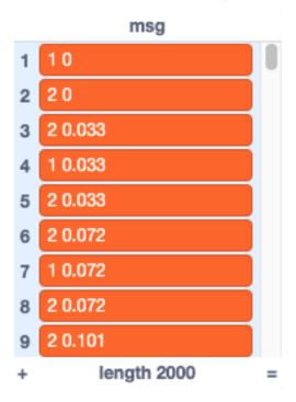
The two processess alternate until index 1500, at that time process 2 has done the 1000 iterations and terminates. Process 1 continues for another 1000 iteration roughly every 33 ms. The total time is 33 seconds.
